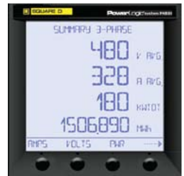
Front panel display showing function selection buttons and 3-phase voltage, current and power summary display.
