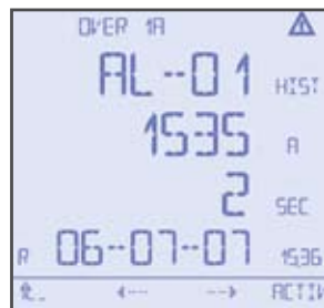
Alarm display showing active alarm
