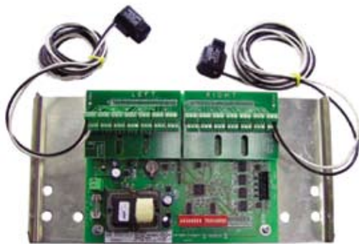
PowerLogic BCMSC split-core branch current monitor, showing two connected CTs (maximum 42 possible), signal acquisition board and mounting bracket.
