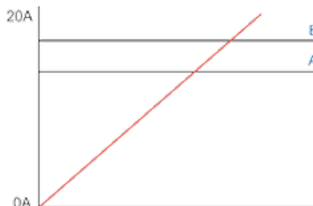
Programmable warning (A) and critical (B) alarm thresholds (example is for 20 Amp circuit).
