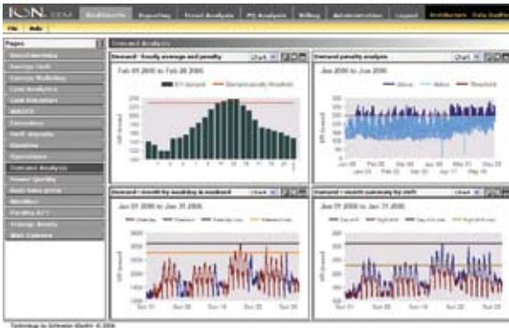
This screen capture is not from the Ford system. It is an example of a PowerLogic ION EEM dashboard screen that depicts similar information to that which is in use at Ford. PowerLogic ION EEM provides access to demand analysis reports that can be viewed hourly, weekly, monthly or customized to best serve energy conservation needs.
