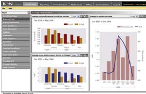
This screen capture is not from the Ford system. It is an example of a PowerLogic ION EEM dashboard screen that depicts similar information to that which is in use at Ford. The browser based PowerLogic ION EEM dashboard provides access to historical utility consumption data for benchmarking production vs. non-production periods to compare similar facilities.
