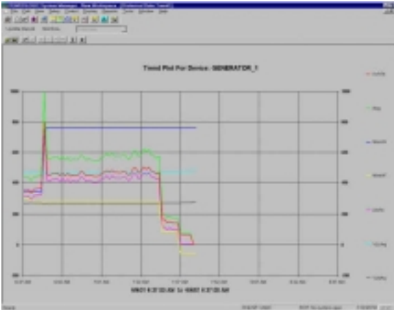
Graph of paralleling system Generator 1 run: Friday morning June 8, 2001
